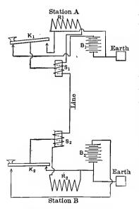
FIG. 173. Differential Duplex Telegraph Circuits.
